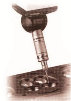
量測運用 SP25M taking points with a TP20 module
